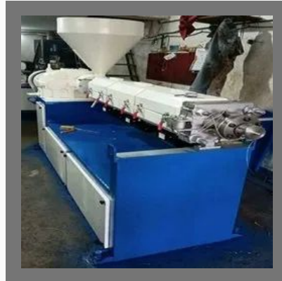
Plastic Pipe Extrusion Line
